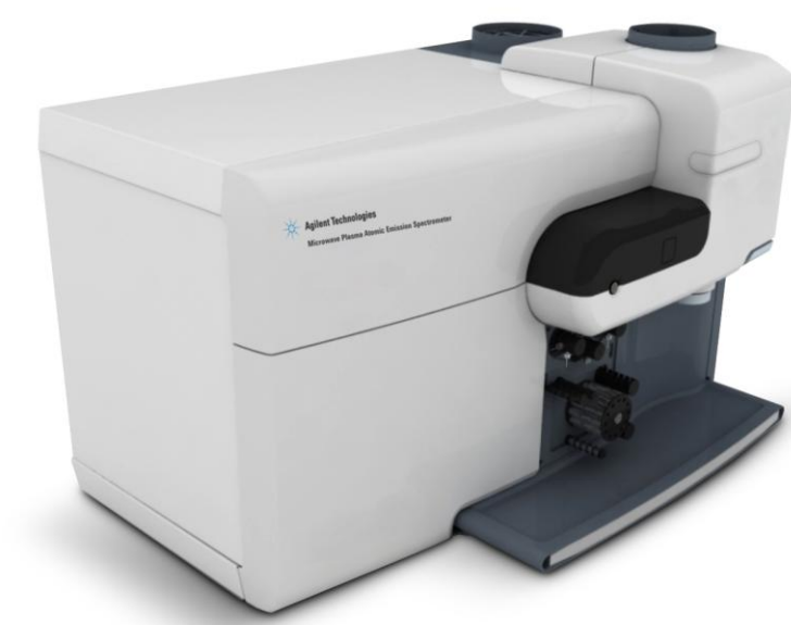
Fig. 1 The Agilent 4100 MP-AES, microwave plasma atomic emission spectrometer.
